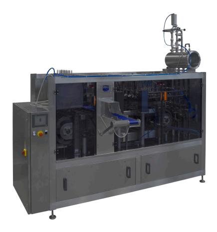
The machine has 9 operating stations and has an electromechanic, pneumatic-assisted functioning. Each station as one function (multiple dosing, labeling, get the top etc). More function permits to have a more flexible machine and packing more type of products. It is realized in AISI304 and it is completed with AISI304 protection covers on the base, aluminium/polycarbonate panels with safety microswitch on the top and adjustable feet or wheels.
