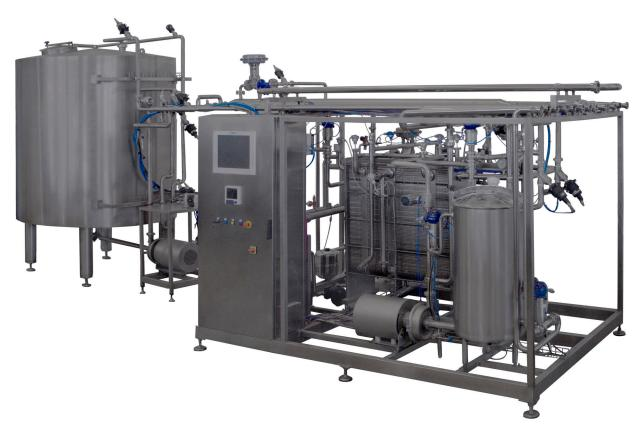
Managed via PLC on HMI with 12 "color touch-screen LCD screen, from which it is possible to check the status of the valves, the state of the pumps, the percentage of opening of the modulating valves, the temperatures, the pressures in real time on P&ID. the instant flow rate, the liters of product processed, the level in the tank, the status of the plc, etc. 10 production recipes are available.
