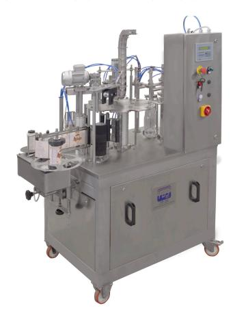
The machine has **5 operating stations** and has an electromechanic, pneumatic-assisted functioning.
