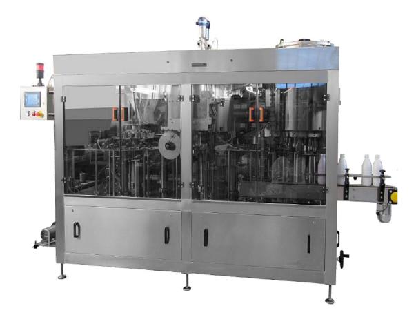
The machine has **8 operating stations** and has an electromechanic, pneumatic-assisted functioning.
