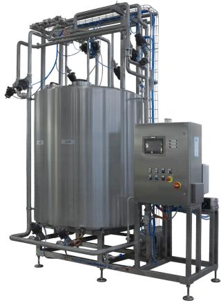
Managed by a PLC on HMI with colours touch screen 12" where is possible to control in real time the state of valves, the state of pumps, the temperatures, the instant flow, the tanks level, the percentage of solutions, the state of PLC, etc.
